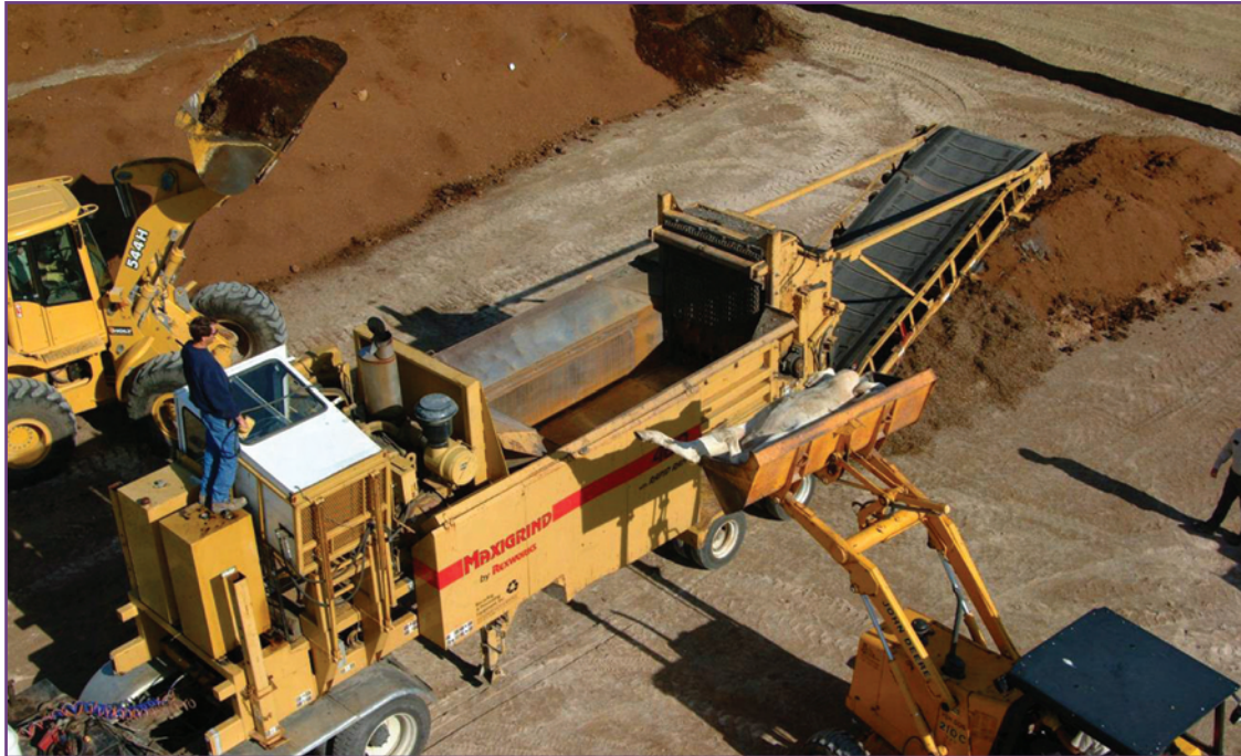
Figure 6. Loading of a carcass into a large-scale carcass grinder and windrows of composted ground carcasses. (Courtesy of Dr. John Kube of Elanco Animal Health, Greenfield, IN)
