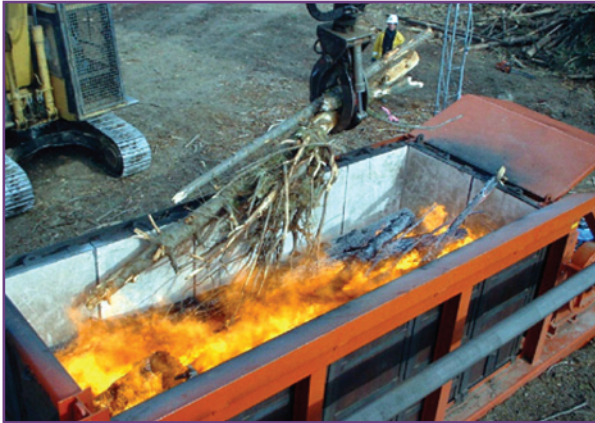
Figure 2. An air-curtain burner with a refractory fire box (left) and a trench (right). (Courtesy of Air-burners, LLC, Palm City, FL)
