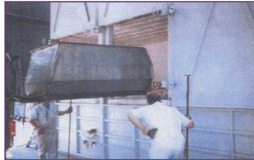
Figure 3. Views of carcass gasifying system used in Scotland for the bovine spongiform encephalopathy crisis. (Photos courtesy of Brookes, BGP, Inc., presented in the North Carolina Disposal Roundtable, Farm Bureau Federation of Raleigh, NC, March 30, 2006)
