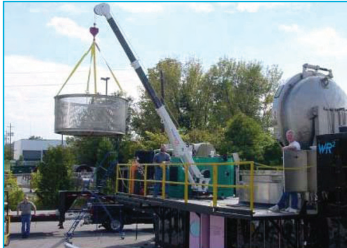
Figure 6. A mobile alkaline hydrolysis unit. (Photo courtesy of Waste Reduction by Waste Reduction, Inc., Indianapolis, IN)
