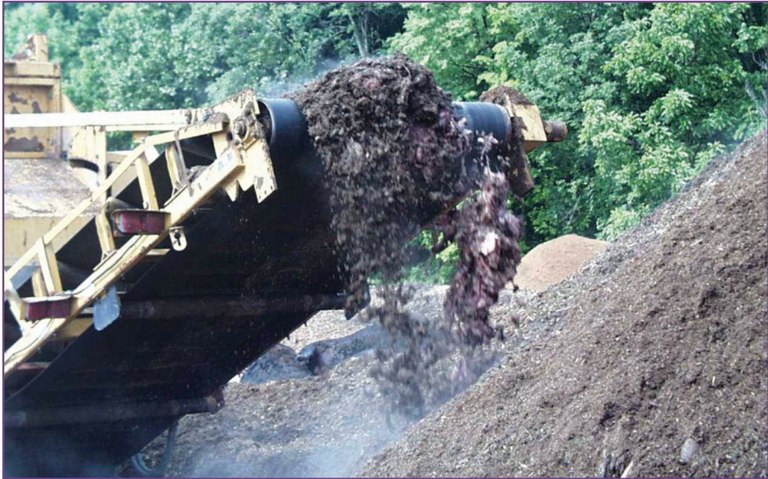
Figure 7. Ground carcass mixed with amendments ready for composting. (Courtesy of Dr. John Kube of Elanco Animal Health, Greenfield, IN)
