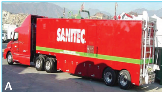
Figure 6. Views of a completely sealed mobile container (A), a mechanical loading system (B), a drop-off container (C), and a front-dump truck (D) used to temporarily store and transport biomass materials ( Courtesy of Kent Munden, USDA-APHIS, Clifton, TX ).
