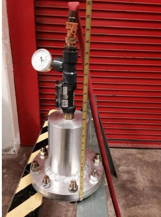
Figure 1. Fluid Containment Assembly
