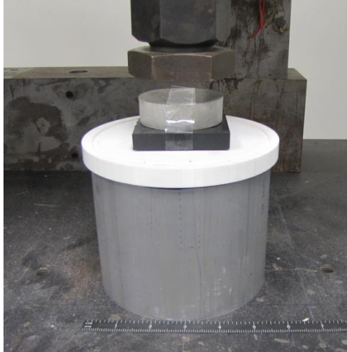
Figure 8: Yield Stress Determination Test Set-Up
