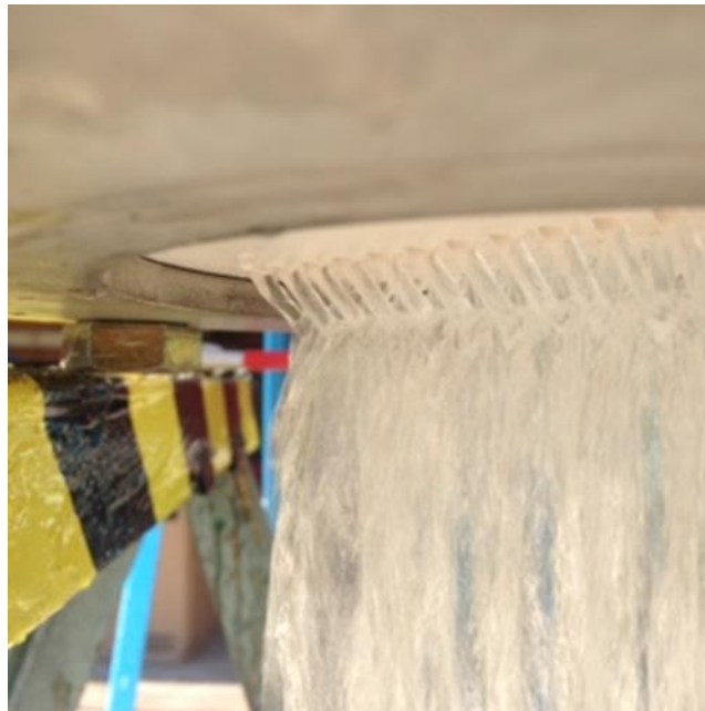
Figure 15. Flow of Water through the Self-Impinging Injector as the Test was Conducted
