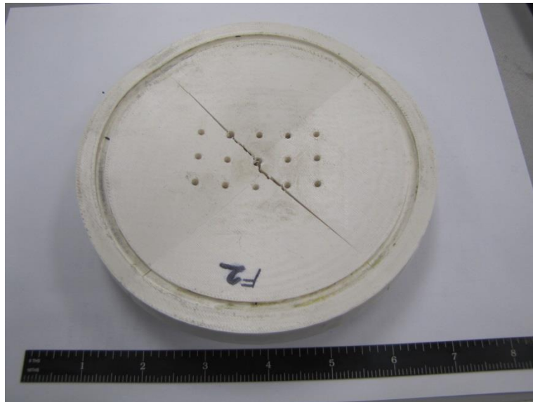
Figure 9: Failure Mode of the Standard Showerhead Injector
