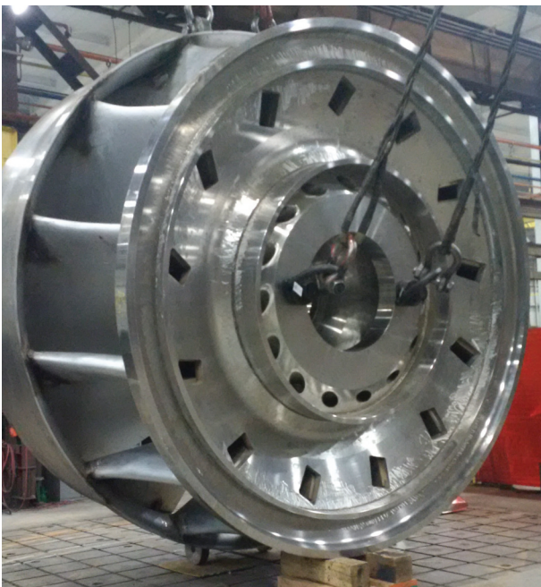
One of the new self-aspirating vented turbines for Center Hill powerplant is assembled at Voith Hydro's York, Pennsylvania manufacturing facility. The turbine has hollow blades enabling ambient air to pass through into the discharge improving downstream water quality and permitting year round operation. Photo:USACE
