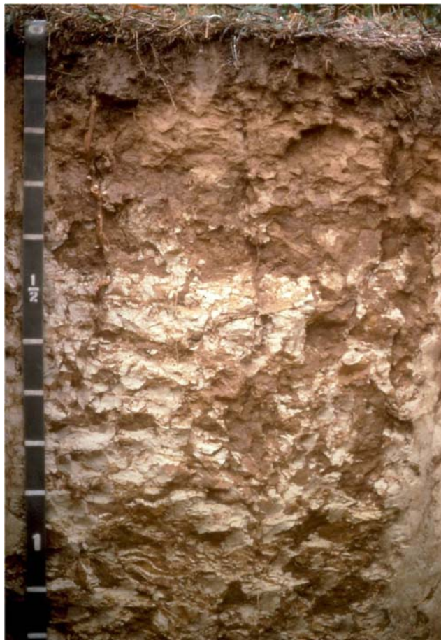
Figure 10-18.—An upland soil formed in material derived from diatomaceous earth. It has a matrix with chroma of 2 below a depth of 18 in (45 cm) and 5YR 4/6 clay films in pores and along ped faces. The colors of the matrix could be misinterpreted as evidence of an aquic moisture regime.
