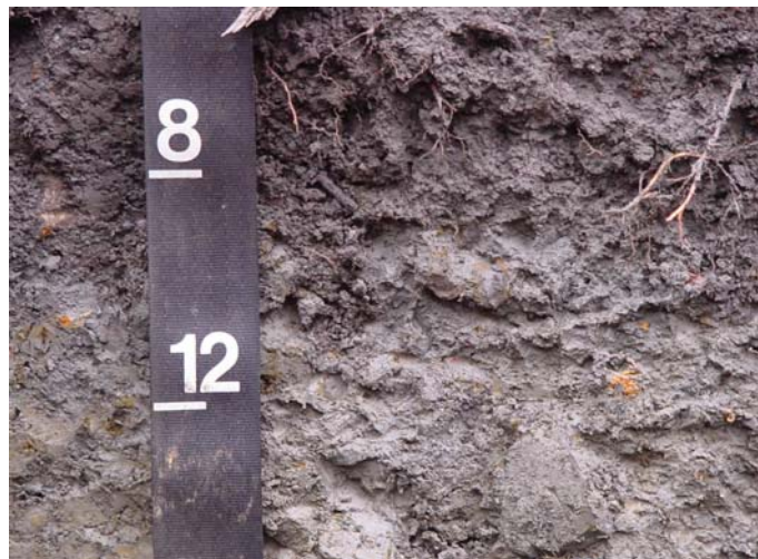
Figure 10-15. —A closeup of burnt shale showing the reddish parachanners and pseudomorphs that can be misinterpreted as redox concentrations.
