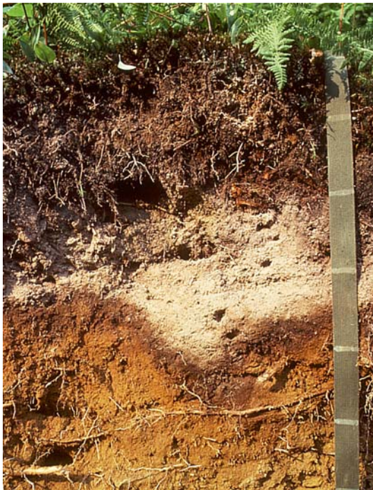
Figure 10-8.—A dry Spodosol with a thick E horizon that could be mistaken for a hydric soil by meeting Field Indicator F3 (Depleted Matrix).
