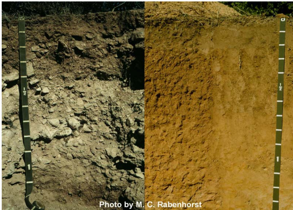
Figure 3-1. —These two soil profiles formed under dramatically different climates. The soil on the left formed under an arid climate (annual rainfall 12 in, or 300 mm) and has a zone of calcium carbonate accumulation in the Bk horizon that extends from 16 to 40 in (40 to 100 cm). The pH in the Bk horizon is approximately 8.1. The soil shown on the right formed in a humid environment (annual rainfall 44 in, or 1,100 mm) where soluble weathering products are quickly leached from the soil. This soil profile has no carbonates present at all. The pH of the Bt horizon, which extends from 8 to 28 in (20 to 70 cm), is approximately 5.5. Scale is in 4-in increments (10 cm).
