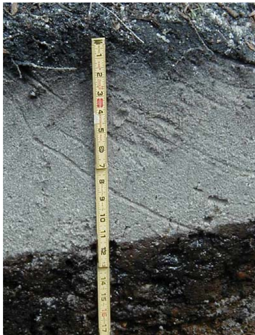
Figure 10-10. —A hydric, coastal plain Spodosol having a gray E horizon with translocated organic matter creating a splotchy pattern throughout the horizon.
