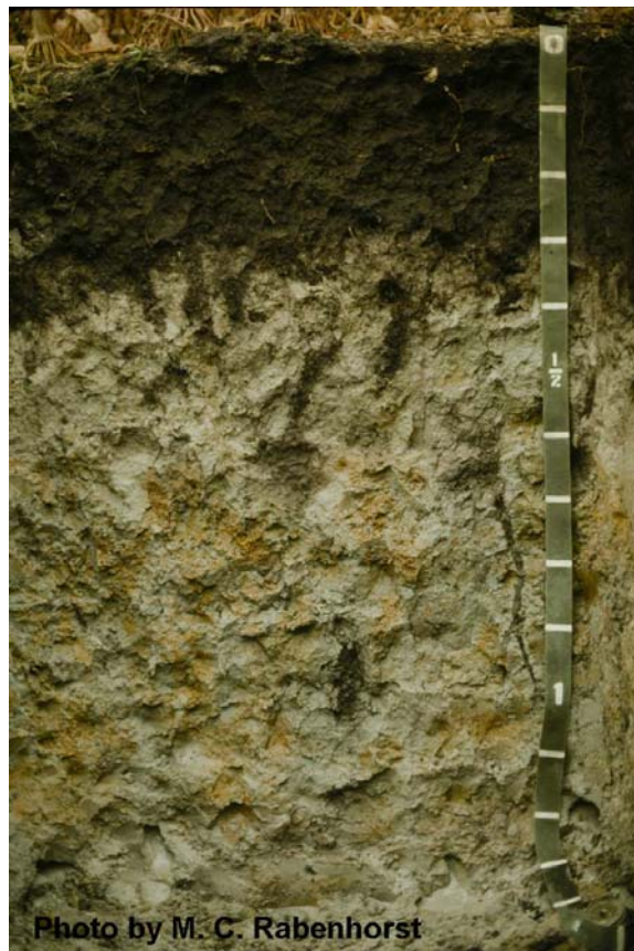
Figure 4-10.—Soil profile from which iron has been largely removed, resulting in a gray Btg horizon.
