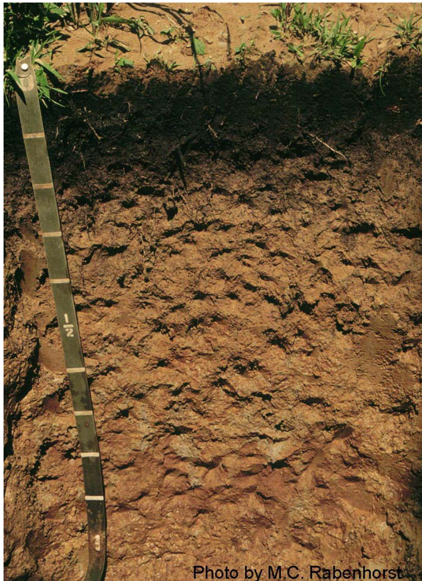
Figure 10-3. —An anomalous, bright, loamy hydric soil from a University of Maryland study site. The typical matrix is 10YR 5/3 or 4/4 at a depth of 8 to 20 in (20 to 50 cm) and 10YR 4/6 at a depth of 20 to 32 in (50 to 80 cm). It has common medium distinct 10YR 5/2 redox depletions and common medium distinct 7.5YR 4/6 redox concentrations, which occur as soft masses.
