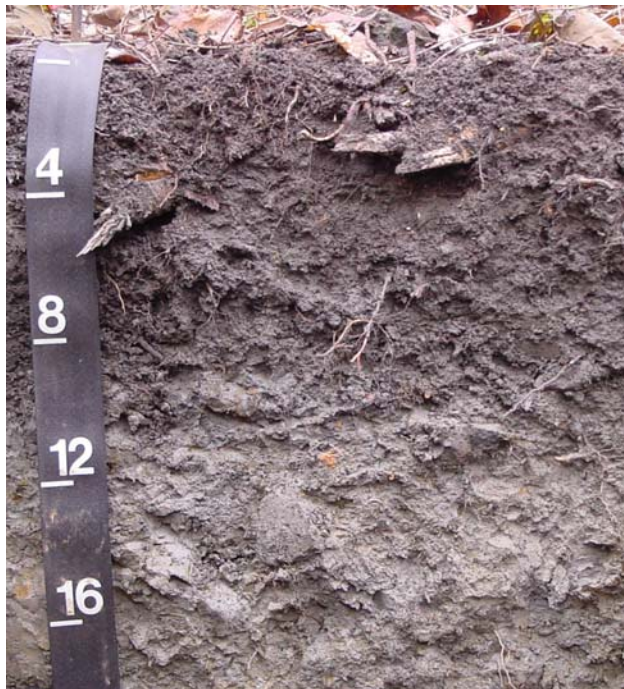
Figure 10-14. —An upland soil formed in material derived from burnt shale on a convex ridgetop. The dark surface layer and the 1-chroma matrix in the B horizon are inherited from the parent material. They could easily be misinterpreted as redox features.
