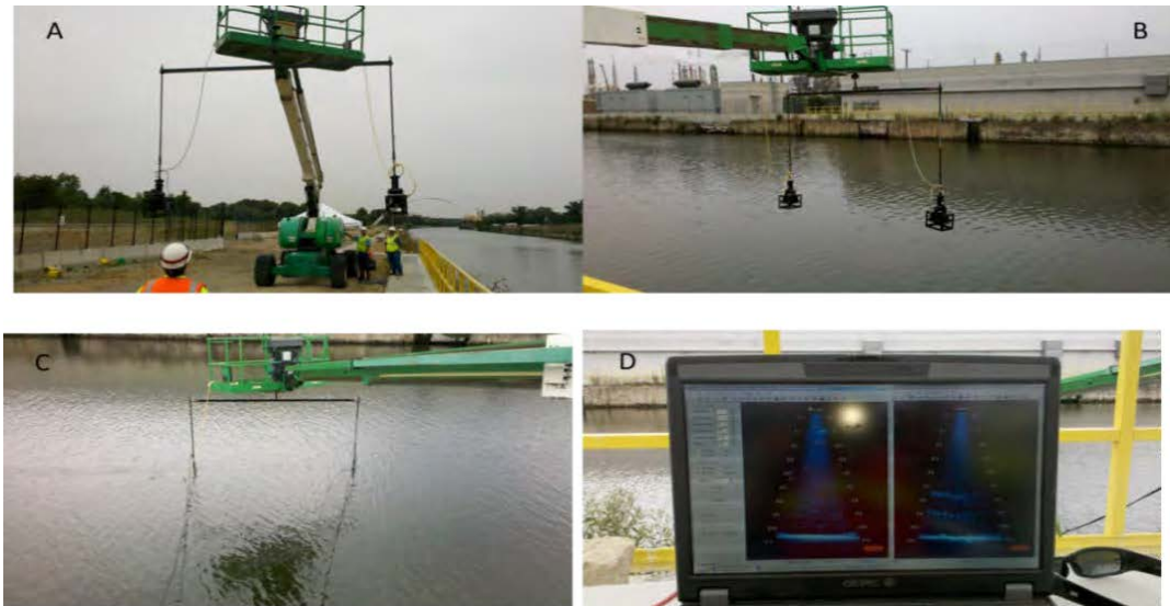
Figure 14. Two DIDSON units being deployed into the CSSC using a telescopic boom lift (A-C) and the two DIDSON units being operated on one computer (D).
