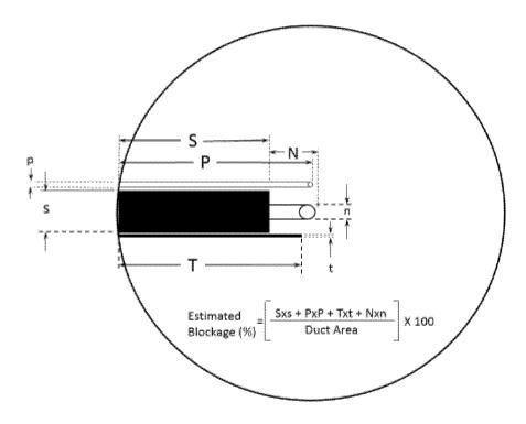
Figure 2-10. Projected-area models for typical pitot tube assemblies.
