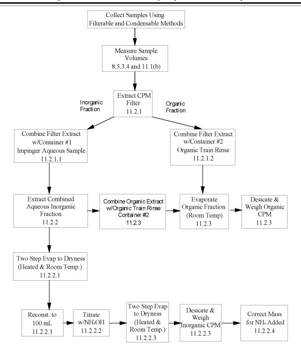
Figure 7. CPM Sample Processing Flow Chart
