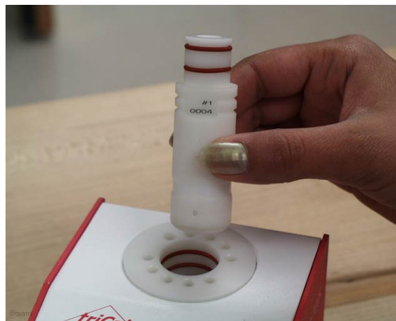
Figures 4-7 and 4-8: Inserting temperature probe and venturi into triCal or tetraCal
