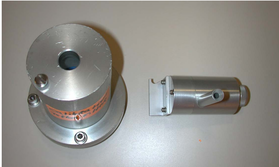
Figure 4-18. Sharp Cut Cyclone Being Inserted into Canister Orifice
