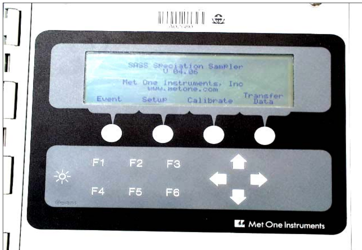
Figure 4-23 MetOne Control Box Displaying Main Menu
