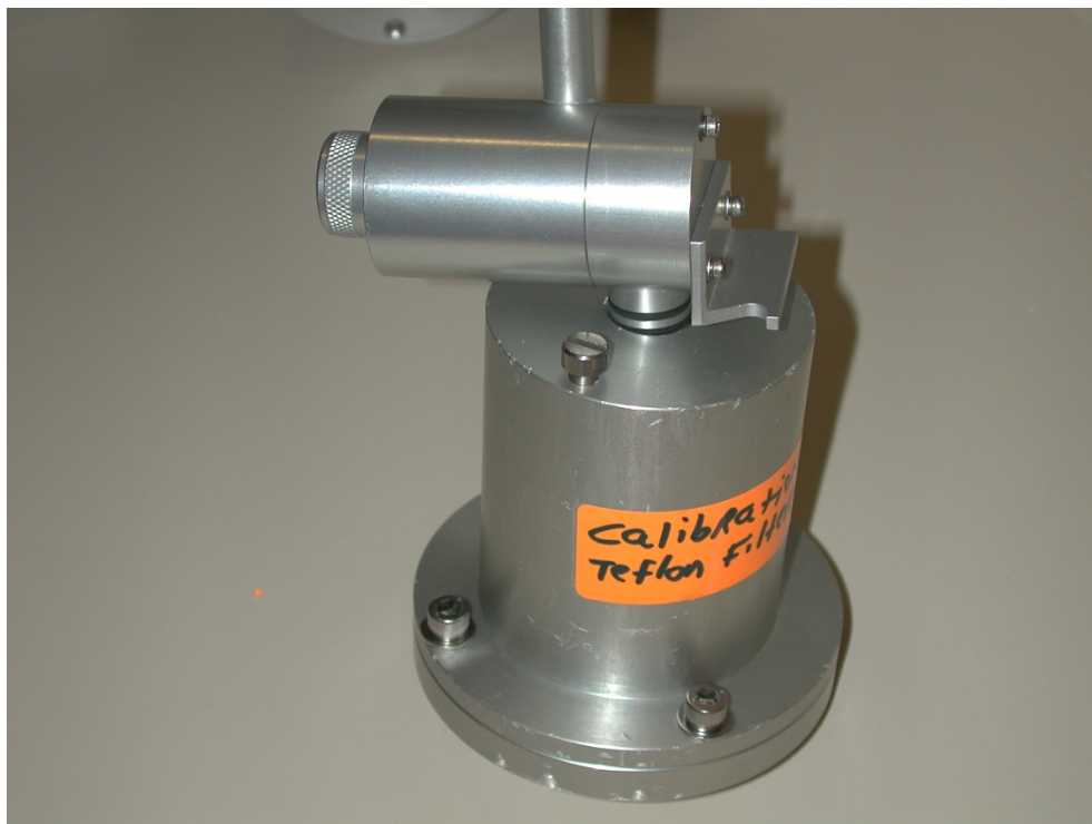
Figure 4-18. Sharp Cut Cyclone Being Inserted into Canister Orifice
