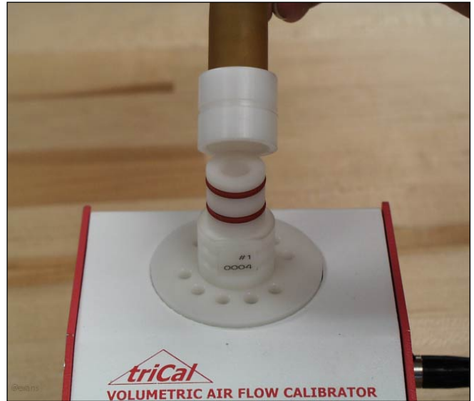
Figure 4-9: Coupling venturi hose adapter with flow measurement tubing
