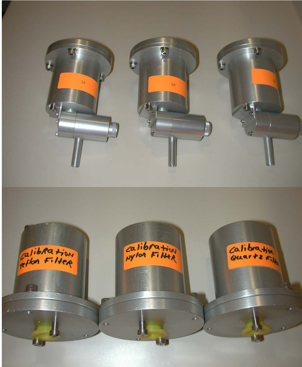
Figure 4.16 Canisters labeled #1, #2, #3, or Teflon®, nylon, and quartz.
