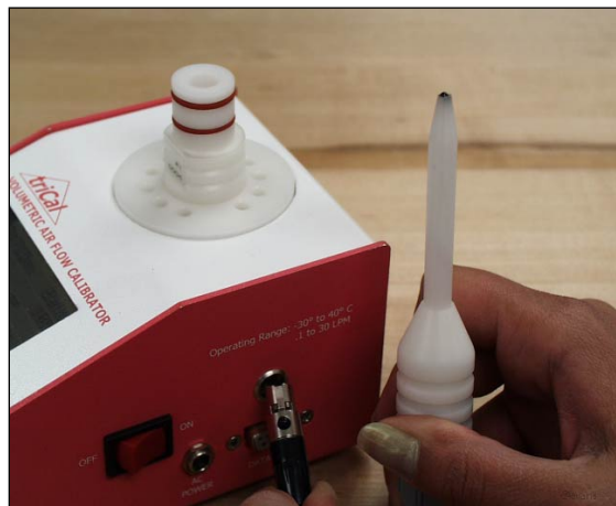
Figures 4-7 and 4-8: Inserting temperature probe and venturi into triCal or tetraCal
