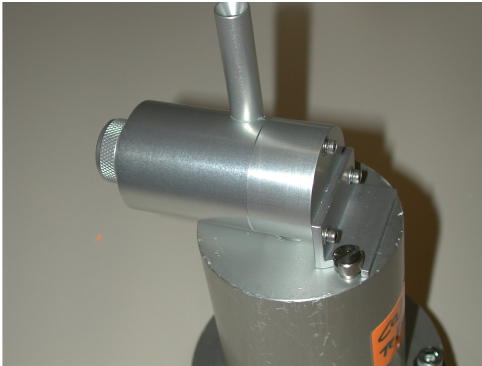
Figure 4-19. Sharp Cut Cyclone fully Inserted into canister orifice and locked in position
