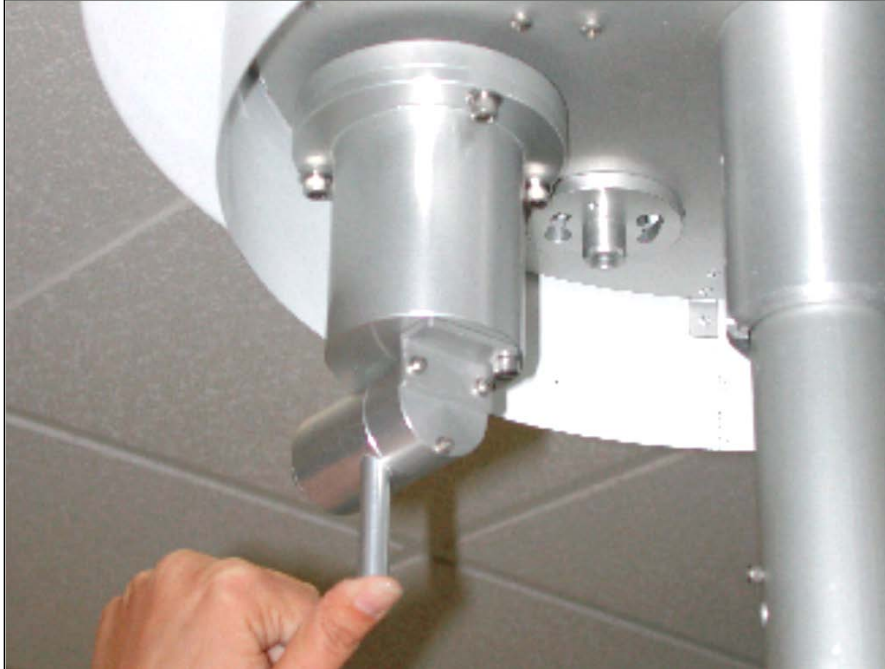
Figure 4-29: Leak check by capping inlet.
