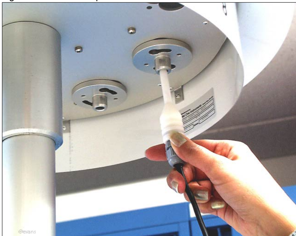
Figure 4-33: Filter temperature audit.
