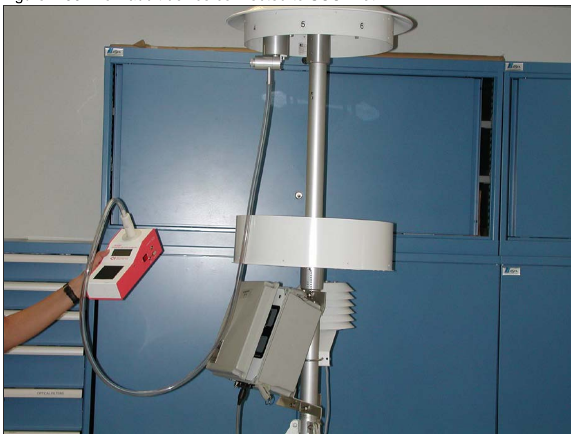
Figure 4-30: Flow audit device connected to SCC inlet.
