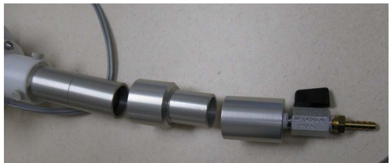
Figure 4-6: Tubing adapter assembly (from a URG 3000N audit kit) can be used for flow checks with deltaCal. Note, BGI sells an adapter that plugs directly into the deltaCal's aluminum downtube.
