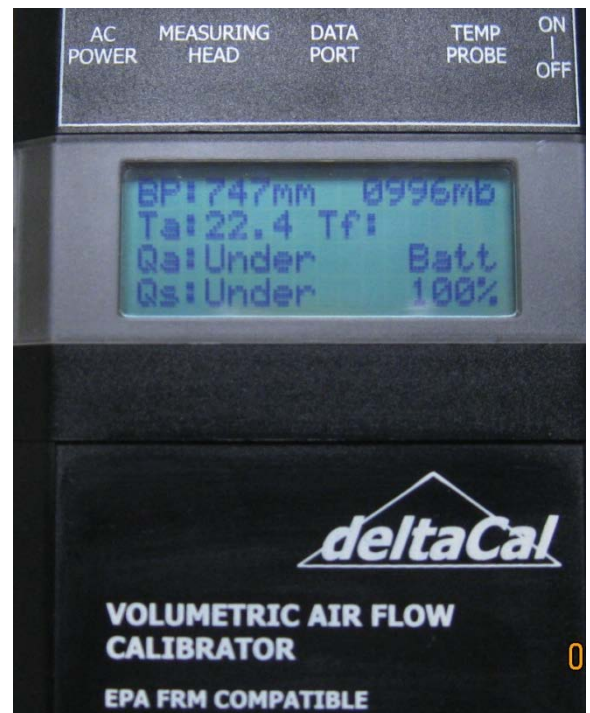
Figure 4-12: Menu screen upon self calibration of newer model deltaCal, triCals, and tetraCal
