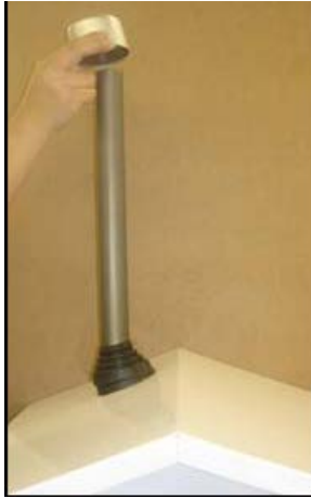
Exhibit 11: Removal of ambient air inlet cap.
