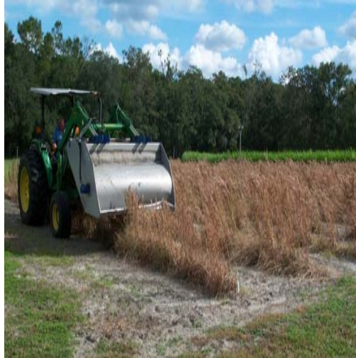
Harvesting Ghost Rider Germplasm with a Woodward Flail-Vac seed stripper
