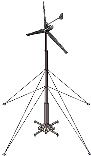
Figure 7: Fully Erected Market Turbine
