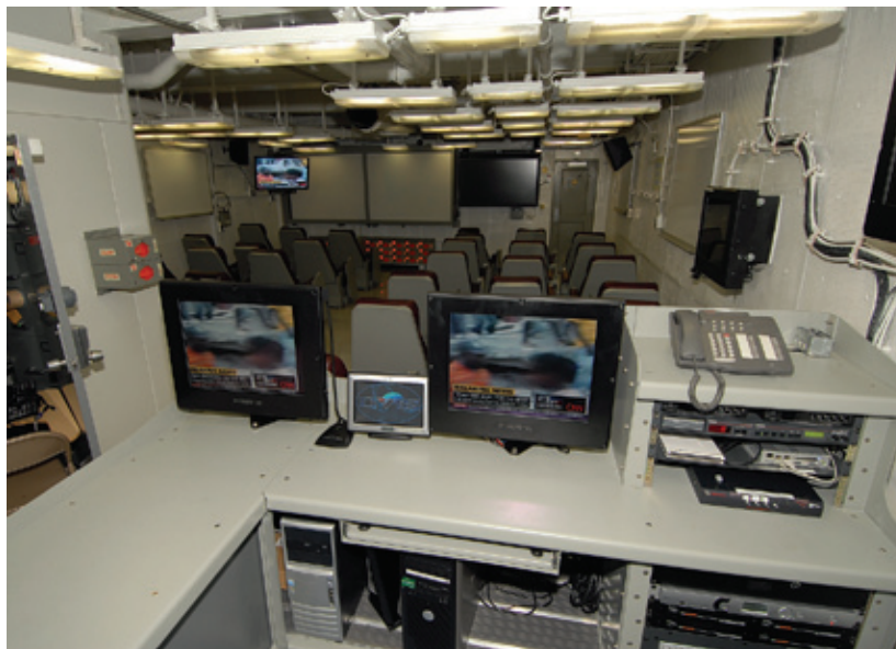
USS GEORGE H.W. BUSH (CVN 77) Ready Room January 2010 with “transformational technology” including updated computer equipment and more robust LAN access. Chalkboards have been replaced by dry erase whiteboards, and paper charts taped to walls have been replaced with LCDs. Photo courtesy of U.S. Navy Strike Planning and Execution Systems Program (PMA 281).
