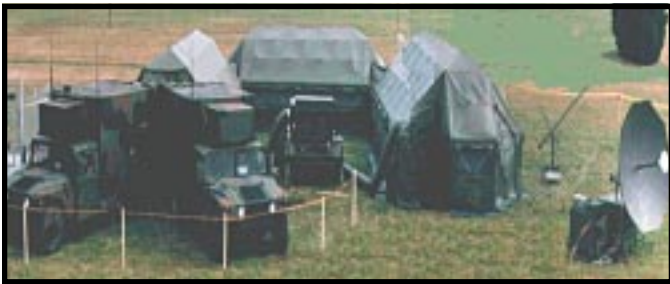
Figure 2. CINCPAC MSQ-126 Fly Away Command Post. The MSQ-126 can deploy via (1) C17, (1) C5 or (4) C130s. It can support a staff of 30 with the full range of DISN services.
