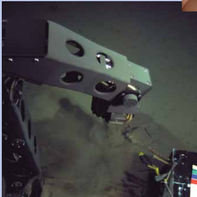
A specialized manipulator arm of the newly built hybrid remotely operated vehicle (HROV)/Nereus samples sediment from the deepest part of the world’s ocean, the Mariana Trench. Photo by Woods Hole Oceanographic Institution.
