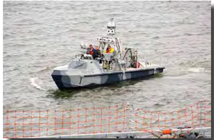
Norfolk, Va. - The Autonomous Maritime Navigation USV intercepts a rogue vessel during a TW09 Sea Trial experiment.
