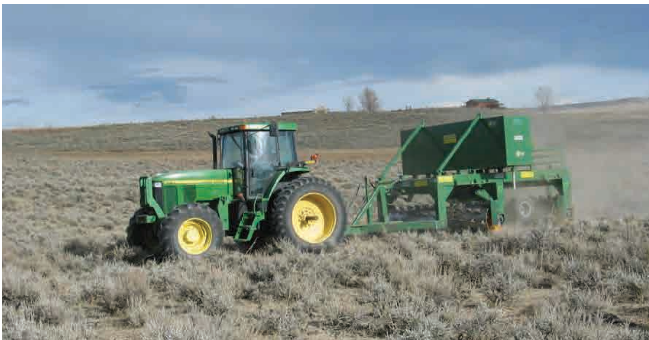
Lawson aerator treating sagebrush to obtain desired conditions. USFWS photo.
