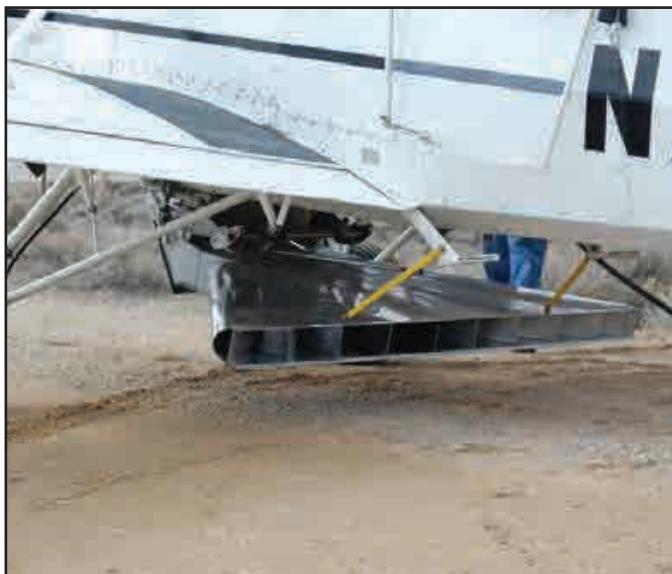
Aerial seeding mechanism(left) and loading the aircraft(right). Photos by Bob Timberman, USFWS.
