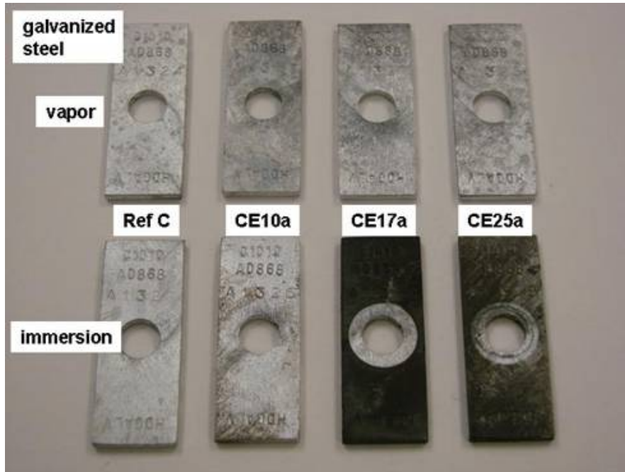
Fig. 18. Post-exposure appearance of the galvanized steel specimens following 28 days of exposure to vapor (~55°C) and liquid (60°C) in the indicated environments.
