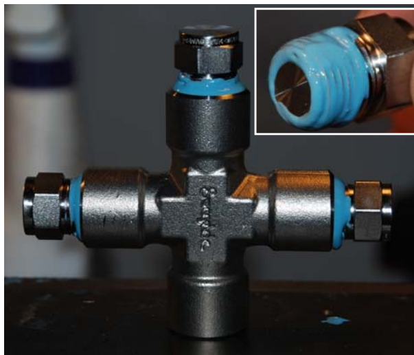
Fig. 12. Thread with applied sealant and the test fixture with three mounted specimens.
