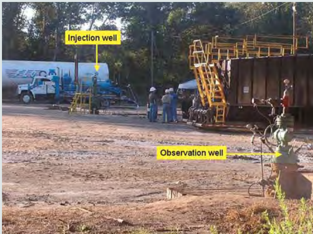
Above and right: Frio Brine Pilot Project: CO 2 injection/observation wells and cross-section schematic.
