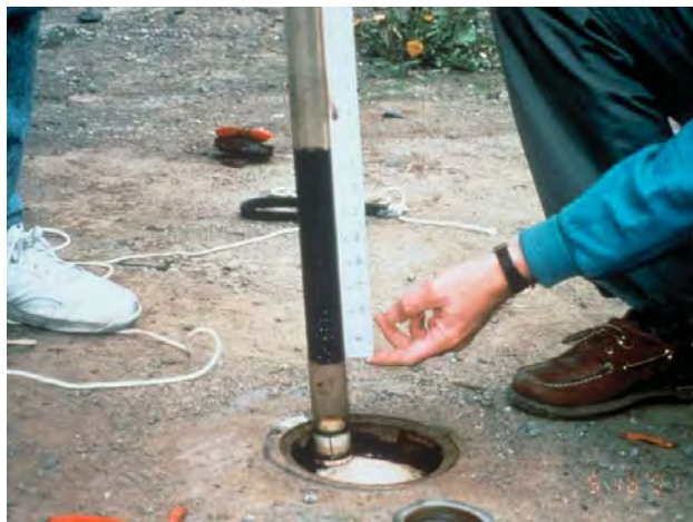
A bailer pulled from a LUST-site monitoring well shows that about a foot of free-product gasoline is present in the ground water.
