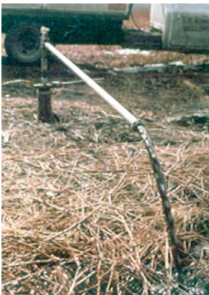
Drinking water wells are rarely as visibly contaminated as the water from this well, which is being pumped to waste, at a former wood treating facility in Minnesota. Routine monitoring is necessary to determine water quality; however, even with monitoring, it is often difficult to pinpoint an actual cause of contamination and many pollutants are not even looked for or assessed.
