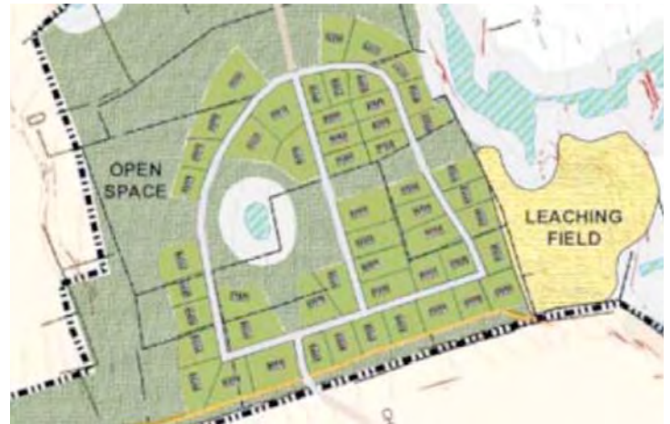
Figure 4. "Community" leaching fields serving multiple single-family homes, with their open space, environmental and aesthetic benefits, are now fully approvable in most states. This plat shows a proposed community leaching field in Connecticut that will be assessed by the Department of Environmental Protection for approval of the hydraulics of the proposed system, the treatment of nitrogen and pathogens, and the mixing of treated wastewater into the area's ground water system. The location of the proposed system's leaching fields, affected soils, the supporting ground water system, and adjacent areas are factors that will influence the design and feasibility of the system.
