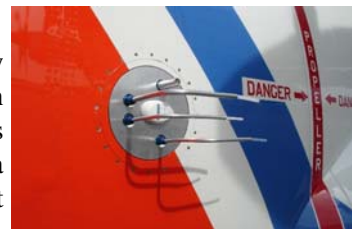
Specially designed window replacement for inlets
