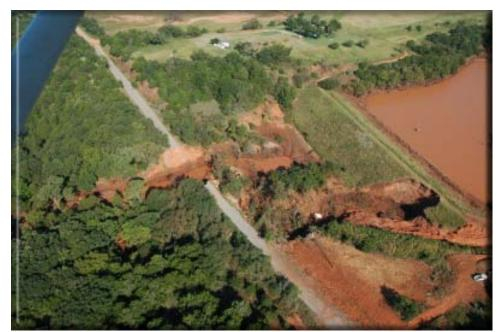
Oklahoma received record rainfalls in 2007. With flooding events, 121 auxiliary spillways flowed, only 20 sustained damage
