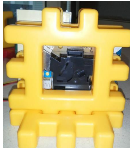
Figure 2. Sensor kit components assembled using a children's building toy pieces and velcro
