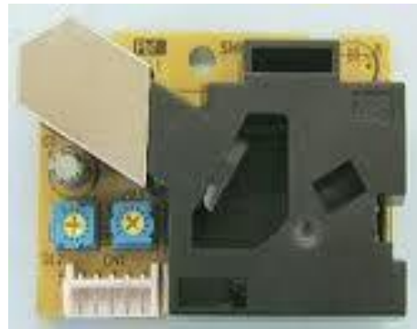
Figure 5. Shinyei particle sensor used in the kit.
