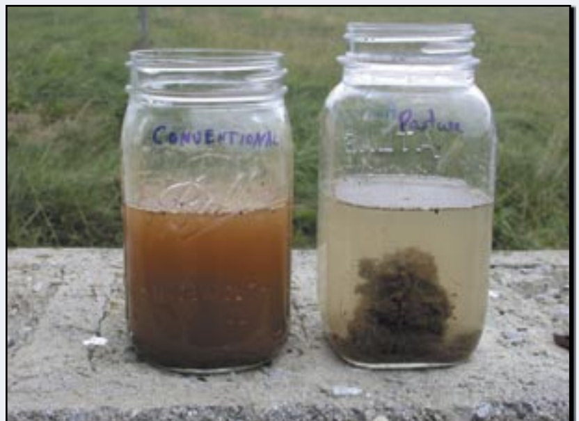
Soil aggregates from pastured fields (right) hold together better than soil aggregates from conventionally tilled fields (left).
