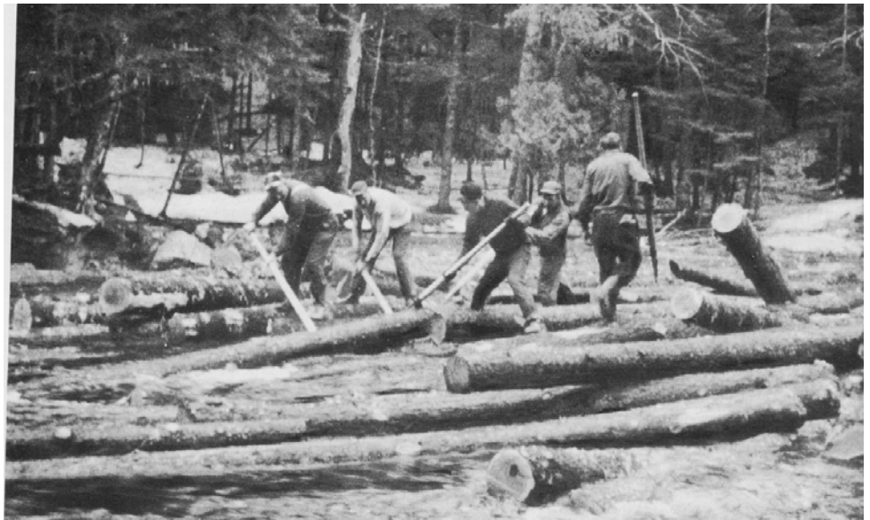
Figure 5. Picture of Crews breaking up a log jam at Grover Pitch “The Pit” on Old Stream with Poles and Peaveys (1965). Photo from (Anonymous 1966).
