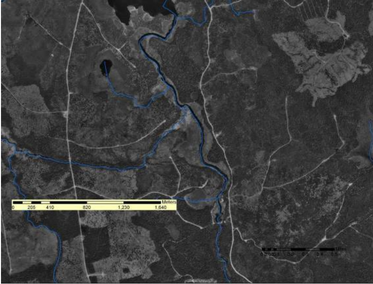
Figure 10. Aerial photography of Canaan Dam to 1 st Lake Old Stream utilized May 1996 gray scale images. Over-widened channel and outline of historic reservoir are apparent in the aerial photography decades after the dam was removed.
