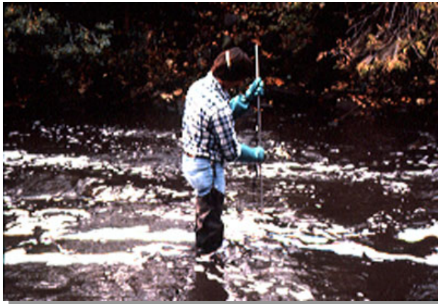
Figure 31: Hand-held current meters are effective devices for measuring velocity, especially in shallow wadable streams.
