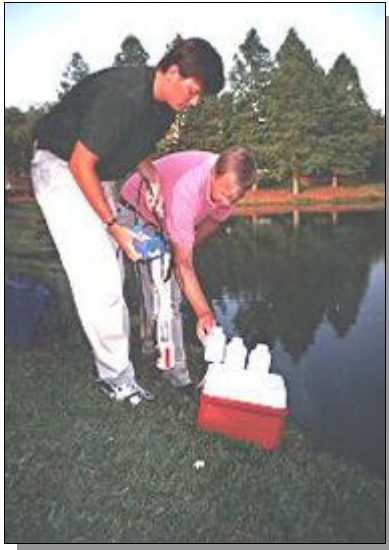
Figure 34: Bottles or plastic containers are used to collect and store water samples that must be transported from the field to the laboratory for analysis. For certain parameters of interest (e.g., metals and nutrients) the sample container must contain preservatives to protect the integrity of the water sample. Proper handling protocol also requires that most sample bottles be placed in ice until they are analyzed at the laboratory.
