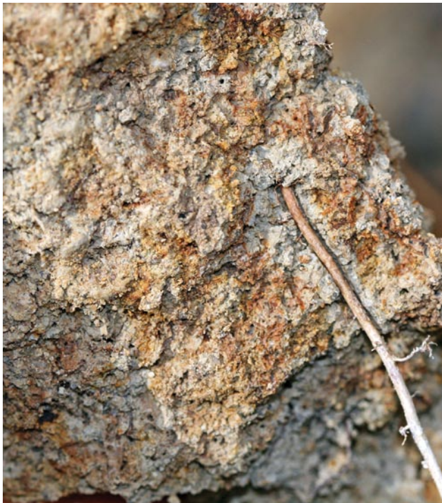
Figure 55.—Redox concentrations occurring as soft masses and pore linings. Also, a redox depletion along a root channel.
