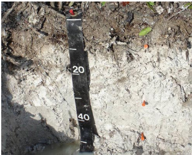
Figure 36.—Indicator F10 (Marl). In this profile, marl begins within 10 cm of the soil surface. The scale is in cm.
