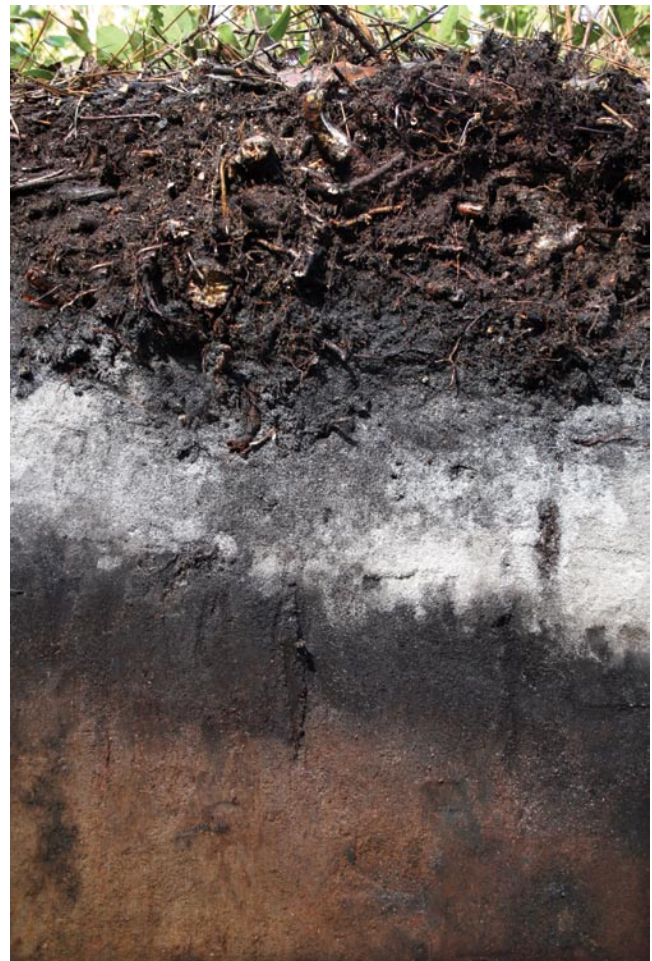
Figure 56.—A wet Spodosol with a splotchy gray and black eluvial horizon above a reddish brown spodic horizon.
