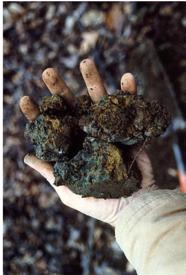
Figure 49. —Glaucanitic soils typically have gleyed, green or black matrices and can have mottles of weathered sulfides that can be mistaken for redox concentrations. If the weathered sulfides in this glaucanitic soil were mistaken for redox concentrations, this nonhydric soil would appear to meet the requirements of indicator F6 (Redox Dark Surface).
