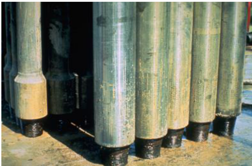
Figure 4-3: Drill Collars Which Provide Drilling Stability and Weight to the Drill String
