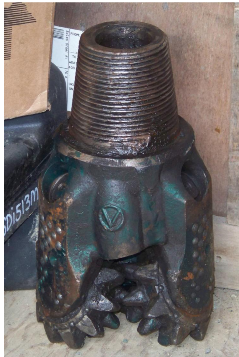
Figure 4-5: Example of Tricone Rotary Drill Bit
