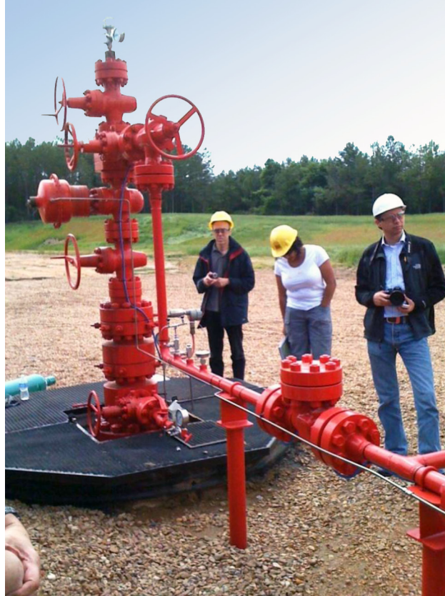
Figure 3-3: Example of an Injection Well
