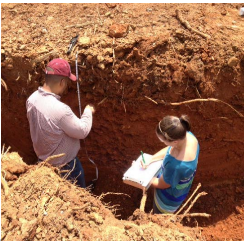
(l-r) Hannah South receives training from Christopher Ford (Soil Scientist) on how to do a soil site investigation for material that will be used to build the core of the pond.
