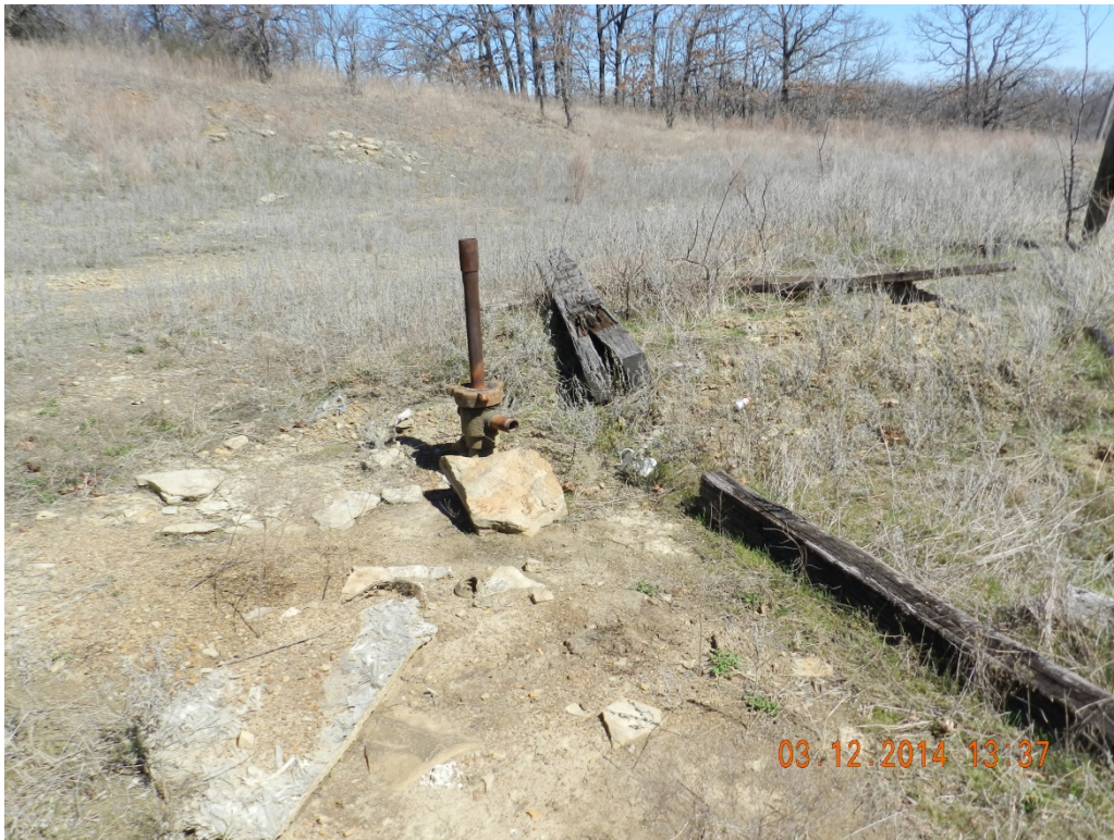
Figure A2-2. Abandoned wellhead at Deep Fork NWR, OK. P Ramirez/FWS Photo
