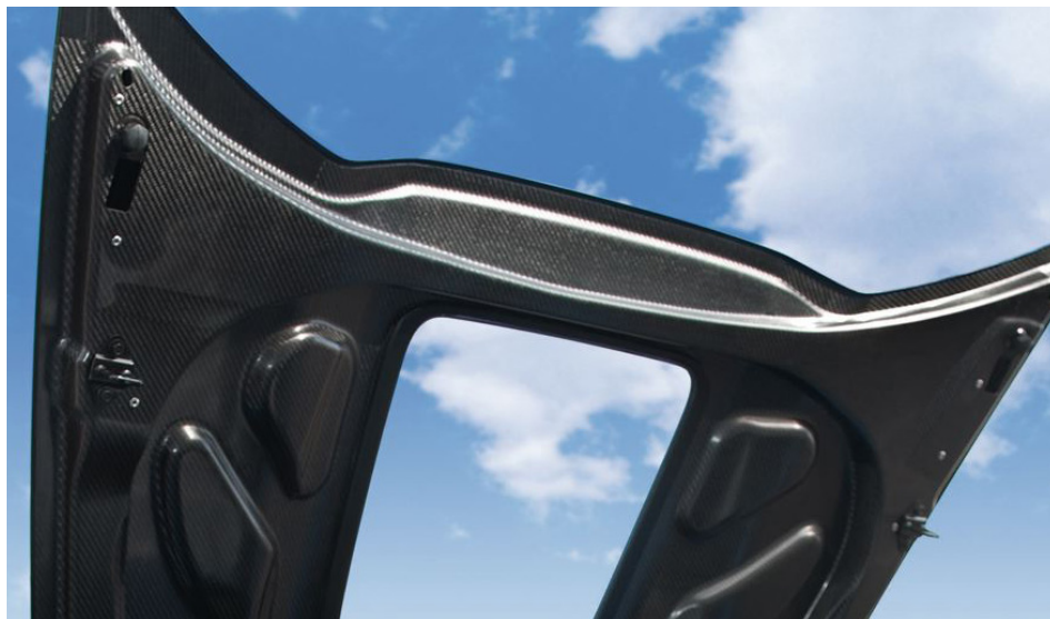
Carbon-fiber composite hood (inner panel) manufactured by Plasan Carbon Composites for the 2013 Chevrolet Corvette ZR1. During manufacturing, a carbon-fabric prepreg (reinforcing fiber and resin) is laid up on a mold and cured with heat and pressure in an autoclave. Photo courtesy of General Motors
