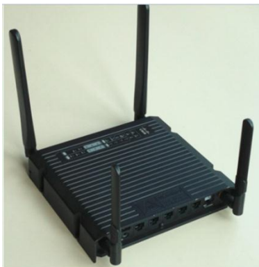
Figure III-38: DSRC radio modem for WPT communications.
