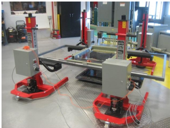
Figure VII-42: Wireless vehicle charging positioning apparatus; 1,000-mm Y and Z actuators, 1,500-mm X-axis actuator.
