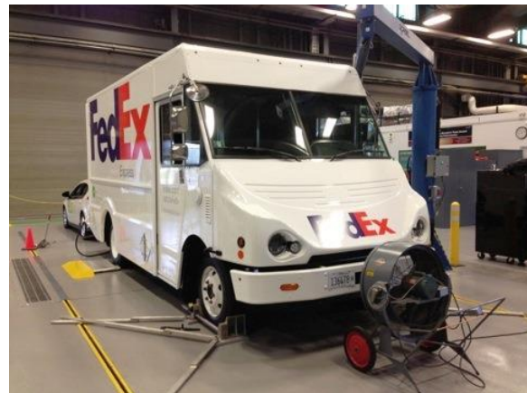
Figure IV-101: Smith Newton EV in Argonne's APRF 4WD testing facility.
