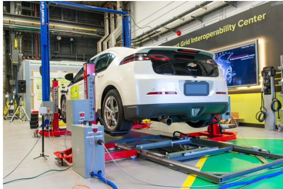
Figure VII-53: Wireless charging vehicle system-level configuration of the positioning apparatus (X, Y, and Z servo amplifiers/safety stops housed in the grey boxes; RF chamber behind).
