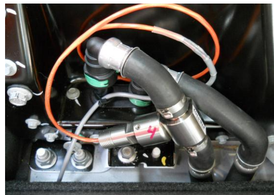
Figure V-142: Example in-line coolant flow sensor.
