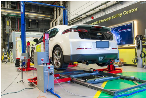
Figure VII-43: Wireless charging vehicle system-level configuration of positioning apparatus. Grey boxes house X, Y, and Z servo amplifiers/safety stops.
