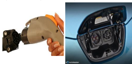
Figure III-24: Conductive charger plug and vehicle receptacle.
