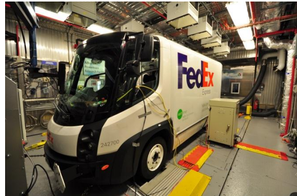
Figure IV-100: Navistar eStar EV in Argonne's APRF 4WD testing facility.
