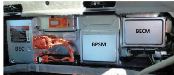
Figure VI-45: Schematic and photo of the Fusion Hybrid's HVTB (Photo credit: John Ireland, NREL).
