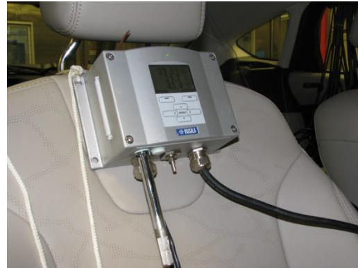
Figure V-140: In-vehicle relative humidity, temperature and pressure sensor.
