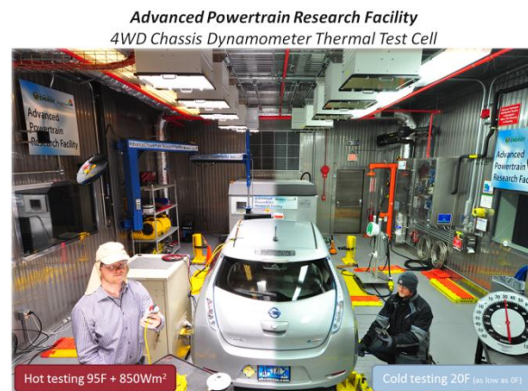
Figure IV-90: Illustration of testing at 95°F with sun emulation (left) and at 20°F cold ambient temperature (right).
