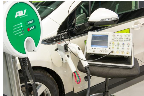
Figure VII-39: Non-invasive interoperability standard (J2953/2) test procedure test point pass-through tool, EVSE, and data collection oscilloscope, ported to a PC via Labview software.
