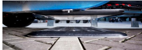
Figure VII-66: Halo IPT wireless charging system interoperability requirement variations in the air gap (flush vs. surface mount).
