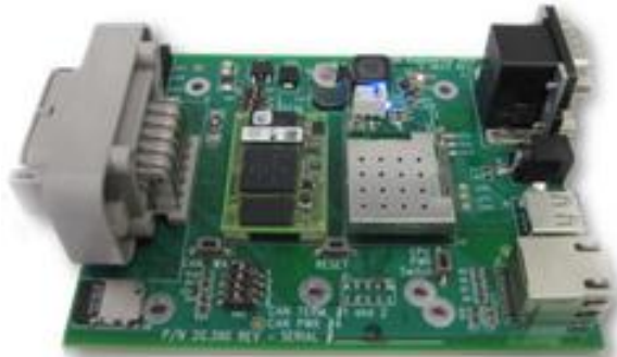
Figure VII-63: Argonne PEV-EVSE off-board charging system communication controller (also can accommodate the proposed IEEE 802.11p standard in J2931/6 wireless charging communication physical layer requirements).
