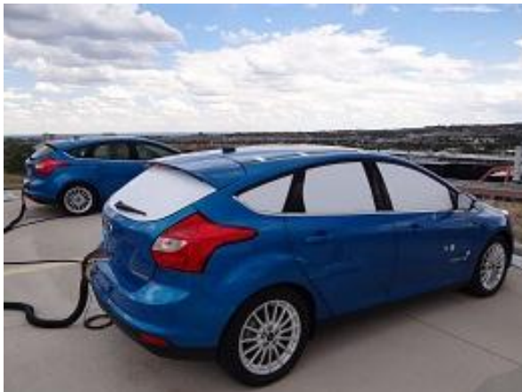
Figure IV-75: Solar load reduction, white film on all glazing.
