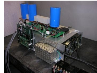
Figure III-16: Wireless power transfer HF inverter (air cooled).
