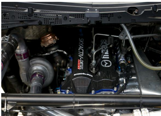
Figure VII-18: Mazda Skyactiv-Diesel production-based race engine captured GRAND AM GX Championship using 100% renewable synthetic diesel fuel (photo by mazdamotorsports.com).
