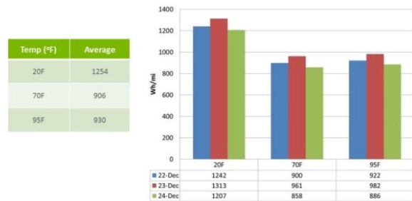
Figure IV-116: Effect of ambient temperature on energy consumption for the Smith EV during back-to-back UDDS/HWY/UDDS cycles (first UDDS cycle is full charge, cold start.) Note: results are estimated, as tests were run at 70°F while operating either the heater or the A/C unit. Additional losses due to powertrain inefficiency at alternative temperatures were estimated and added.
