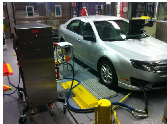
Figure VI-31: 2011 Ford Fusion Thermal Testing Mule. (The thermal testing cart is shown in the lower left-hand corner.)
