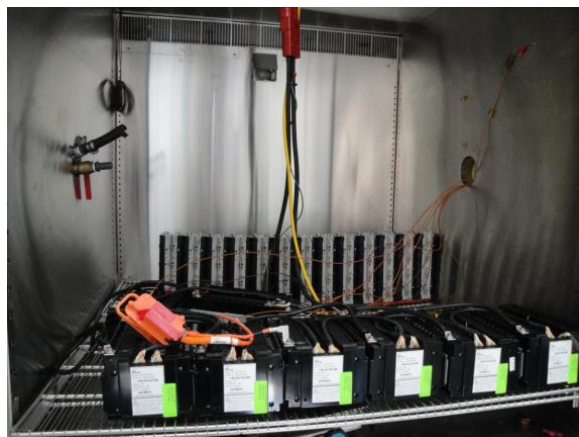
Figure VI-48: JSR LIC modules in an environmental chamber during bench testing, with the production 2012 Fusion Hybrid NiMH modules in the background (Photo credit: John Ireland, NREL).
