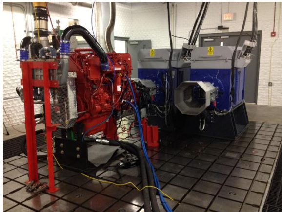
Figure VI-24: Cummins ISX configured for engine-in-the-loop testing.
