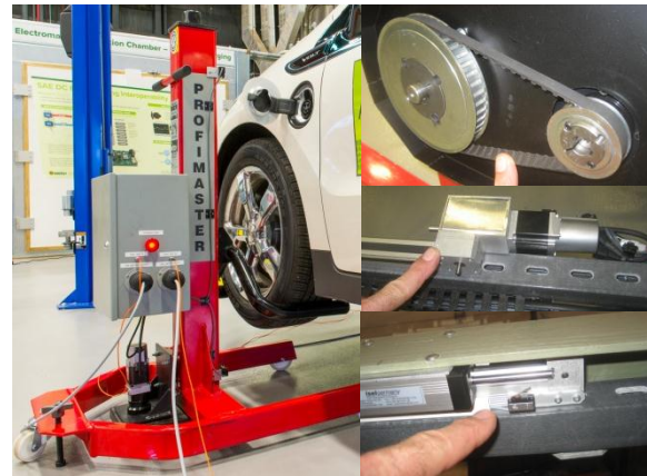
Figure VII-55: Wireless vehicle charging positioning apparatus safety and reliability features: stop screw, interlocks, limit switches, and upgraded gearbox servo systems (1-mm accuracy).
