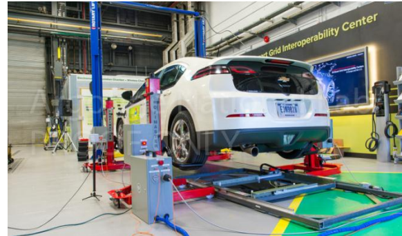
Figure VII-27: Argonne Wireless Charging System Test Fixture.
