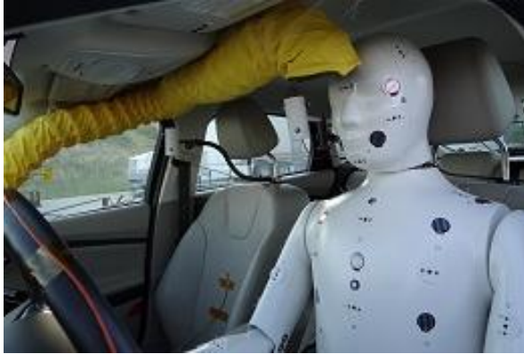
Figure IV-74: Zonal vent configuration with HVAC Manikin.
