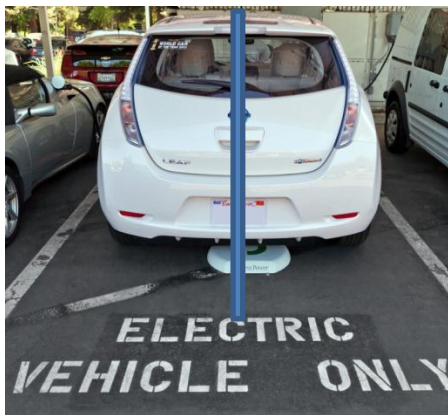
Figure VII-57: Example of the magnetic center of the wireless charging apparatus (not the same as the mechanical center, with respect to setting zero reference on the positioning fixture).
