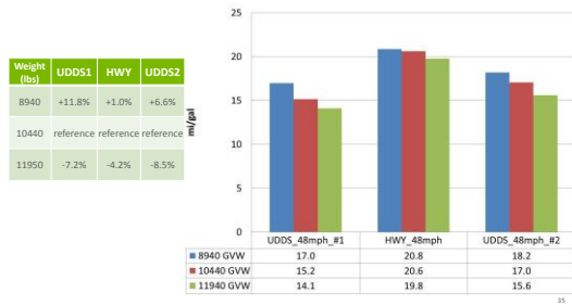
Figure IV-105: Back-to-back UDDS/HWY/UDDS tests at three weights.
