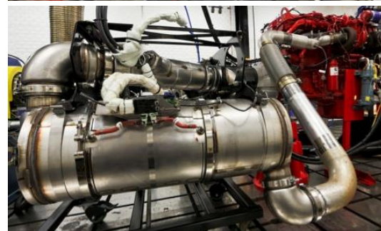
Figure VI-20: Cummins ISX 15L engine and associated exhaust aftertreatment procured for use during experimental phase of Meritor DMHP testing.
