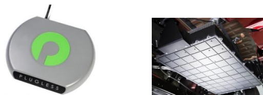
Figure VII-62: Evatran wireless charging system hardware with Bluetooth communication between stationary and vehicle side electronics (open-loop interaction with the vehicle/CAN).
