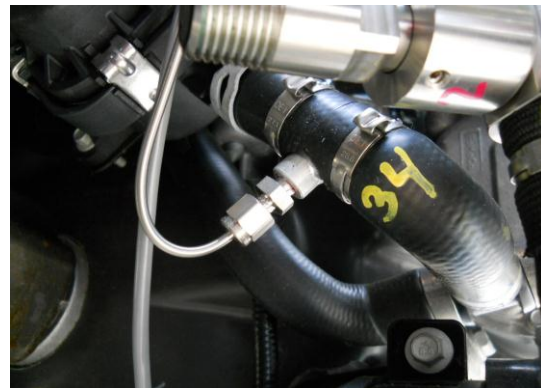
Figure V-141: Example coolant temperature sensor installation.
