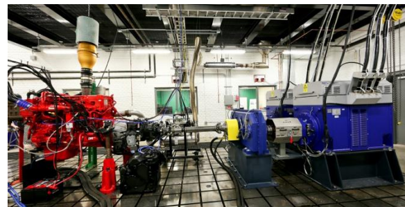
Figure IV-193: ORNL VSI Powertrain Test Cell “power pack” test configuration for heavy duty applications.
