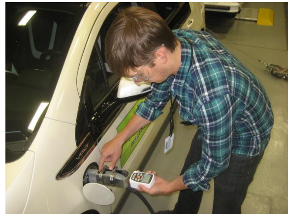
Figure VII-40: SAE J2953/2 test procedures for PEV interoperability-mechanical insertion force measurements.
