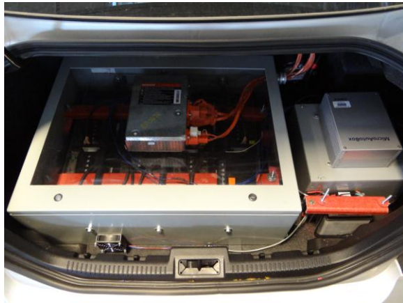
Figure VI-51: Fully integrated conversion system mounted in the trunk of the Fusion Hybrid test platform (Photo credit: Jon Cosgrove, NREL).
