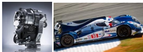
Figure VII-16: Flybrid system employed in #16 Dyson/Mazda (photo by Eric Gilbert Motorsport.com).
