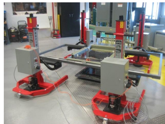
Figure VII-52: Wireless vehicle charging positioning apparatus (1,000-mm Y and Z actuators; 1,500-mm X-axis actuator).
