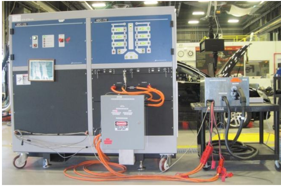
Figure VII-25: SAE DC Charging Test System Utilizing ABC-170.
