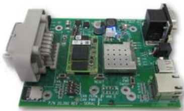
Figure VII-68: Argonne communication controller platform (SpEC module).
