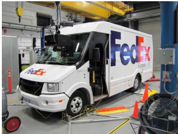
Figure IV-102: Isuzu Reach diesel benchmark in Argonne’s APRF 2WD testing facility.
