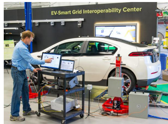
Figure VII-59: Wireless charging positioning apparatus with Narda EHP-200 field probe (next to cart) and FLIR E60.
