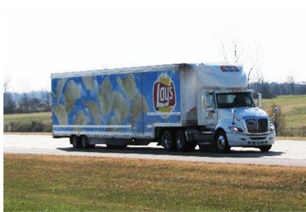
Frito Lay trailer with a Freight Wing gap fairing
