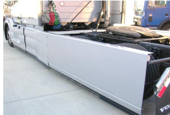
Figure III-14: Prototype Tractor Wheel Skirting Installed on VEV-1.
