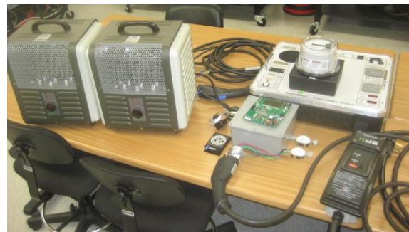
Figure VII-44: NIST Handbook 44 reference proof-of-concept field verification of electricity as a fuel-dispensing system.
