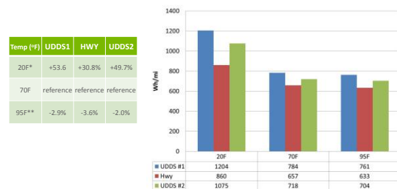
Figure IV-111: Effect of ambient temperature on energy consumption during back-to-back UDDS/HWY/UDDS cycles. (First UDDS cycle is full charge, cold start.)
