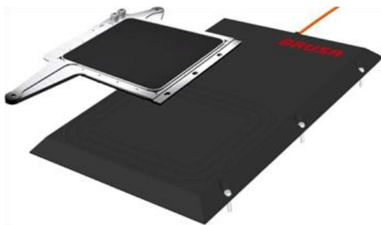
Figure VII-64: Commercial product (Brusa Electronics) self-contained 3.7-kW power electronics and electromagnetics with IEEE 802.11p wireless vehicle-charging communication.
