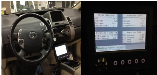
Figure III-37: HMI display of battery pack data in Prius Hymotion.
