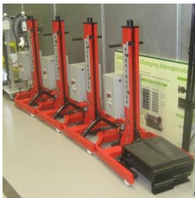
Figure VII-54: Wireless vehicle charging positioning apparatus in storage/transport mode (stacks compactly; self-contained).
