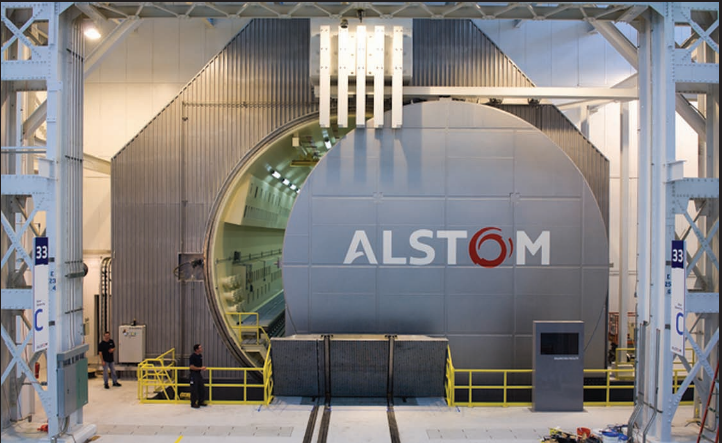
The balancing facility at Alstom's turbine manufacturing facility in Chattanooga, Tenn. Photograph courtesy of ALSTOM.
