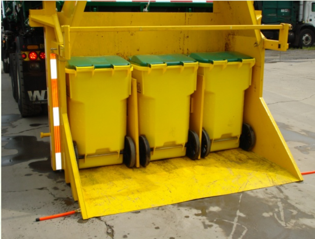
3-65 gallon toters in cart dumper
