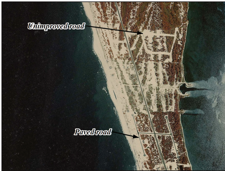
Figure 31. Historic imagery of Florida Unit P30 shows that the subdivision to the north did not have paved roads and therefore did not have a full complement of infrastructure. However, the subdivision to the south did have paved roads. Additional research would be necessary to determine if this subdivision had the other components necessary to constitute a full complement of infrastructure.
