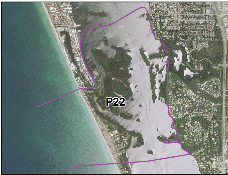
Figure 24. CBRS units are generally left open on the seaward side and are intended to contain the entire sand-sharing system, including the beach, shoreface, and offshore bars. The offshore extent of the units is generally not delineated on the CBRS maps.
