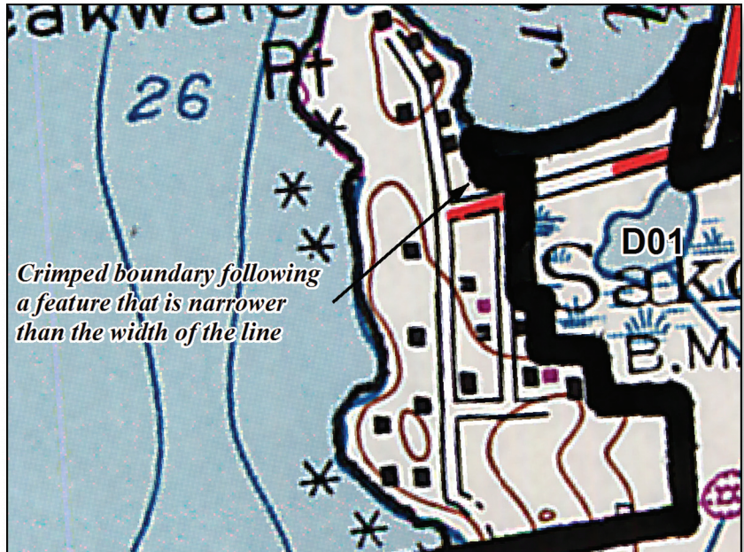
Figure 6. CBRs boundaries on the 1990s era maps can be difficult to interpret because they are typically about 80-100 feet wide on-the-ground. This 1990 map for Rhode Island Unit D01 shows a boundary segment that is about 165 feet wide in one area.
