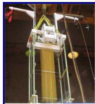
Testing one of SuperPower's FCL modules
