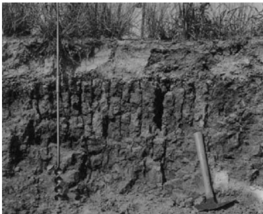
Figure 4.5 Prismatic—the individual units are bounded by flat to rounded vertical faces, distinctly longer vertically.
