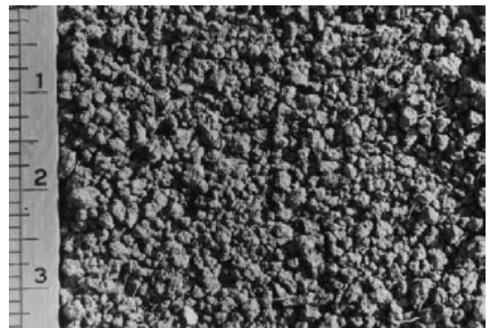
Figure 4.8 Granular—The units are approximately spherical or polyhedral and are bounded by curves or irregular faces.
