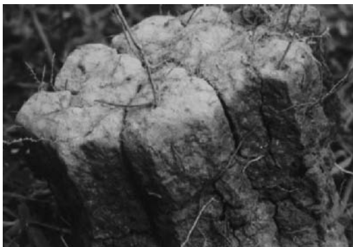
Figure 4.6 Columnar—the units are similar to prisms and are bounded by flat or slightly rounded vertical faces, that have tops very distinct and normally rounded.
