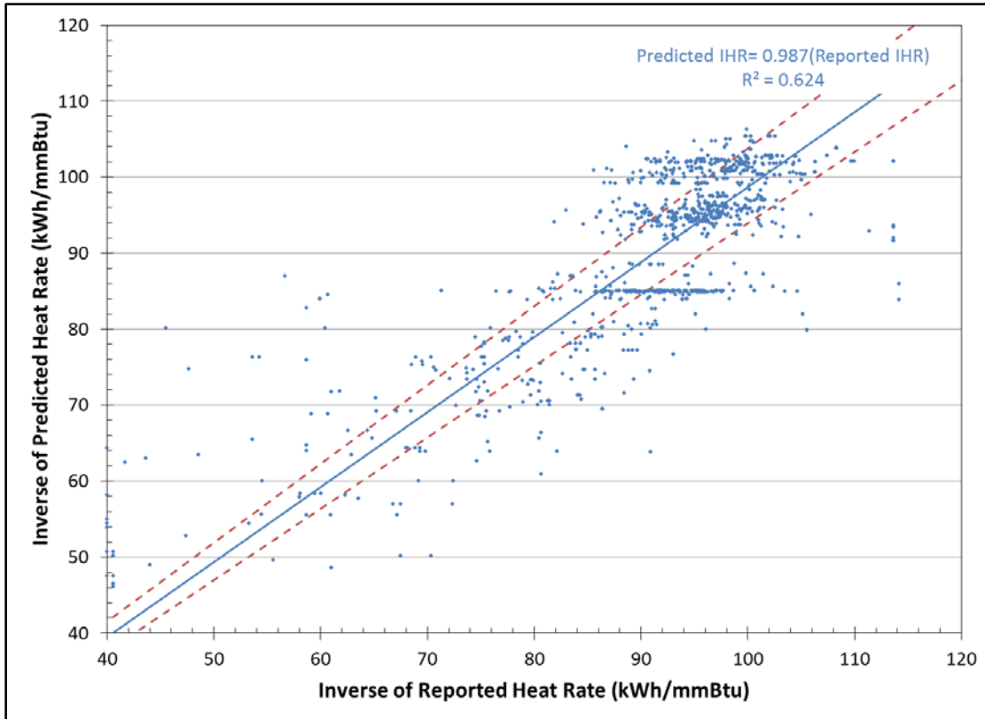
Figure ES-1. Comparison of Reported and Predicted Inverse Heat Rates for All Coal-Fired Generators
