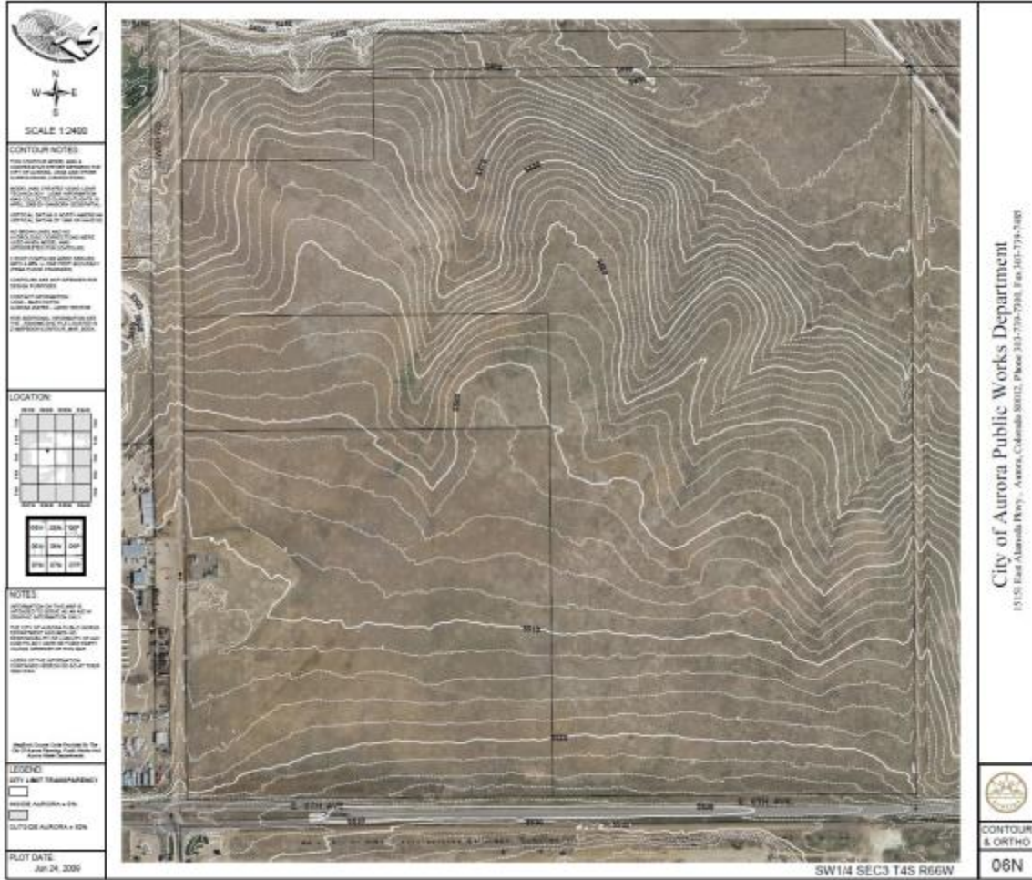
Figure 7. A topographical map of the feasible area for PV at the Tower Road site. Illustration from the City of Aurora
