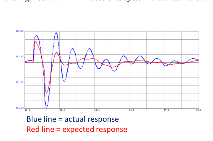
Figure 4: BPA detected power system stabilizer failure at a large hydropower generator using PMU recordings (Source: BPA)
