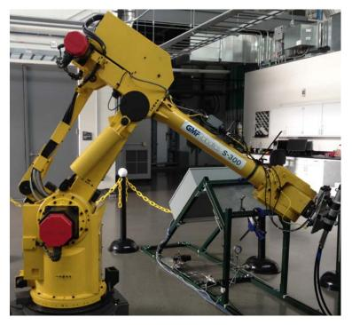
NREL's goal is to run hydrogen hoses through tens of thousands of fill cycles to see how they withstand repeated use—and with its autonomous functionality, the fueling robot makes this kind of long-term, accelerated testing as simple as pushing a button. Photo by Devonie McCamey, NREL 28806
