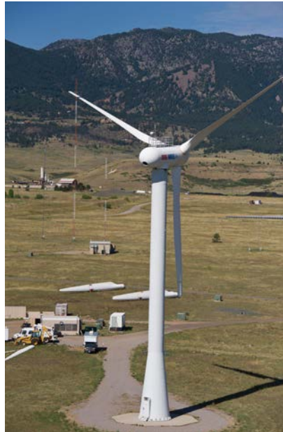
The research team performed automatic generation control and primary frequency control field tests at the NWTC using the 650-kilowatt 3-Bladed Controls Advanced Research Turbine. Photo by Dennis Schroeder, NREL 21893
