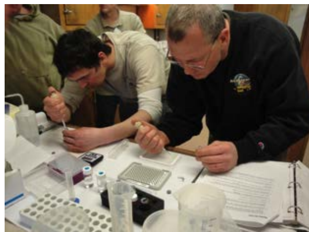
Image 6.1. Fishermen testing for paralytic shellfish poisoning toxins onboard a fishing vessel as a part of the Onboard Screening Dockside Testing biotoxin control strategy (Photo courtesy of Stacey DeGrasse, FDA)
