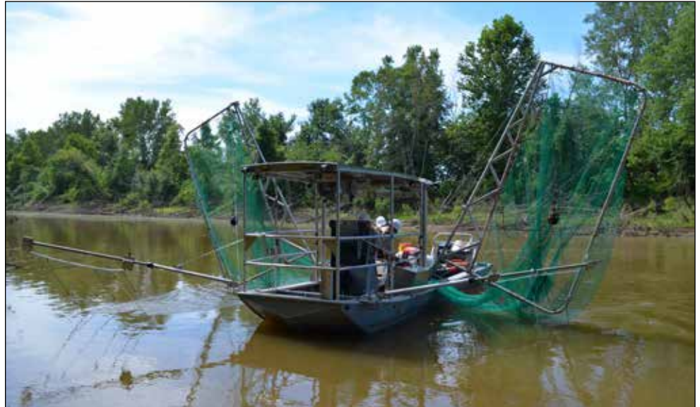
When not in use, the Paupier nets on the Magna Carpa lift out of the water like wings. Katie Steiger-Meister, USFWS
