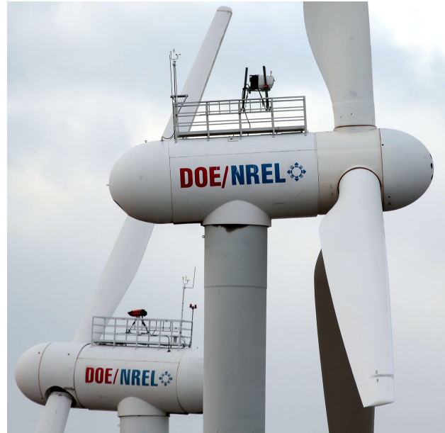
Fig. 1. Lidars mounted on two- and three-bladed research wind turbines at the National Wind Technology Center. (Photo by Lee Jay Fingersh, NREL 32910)
