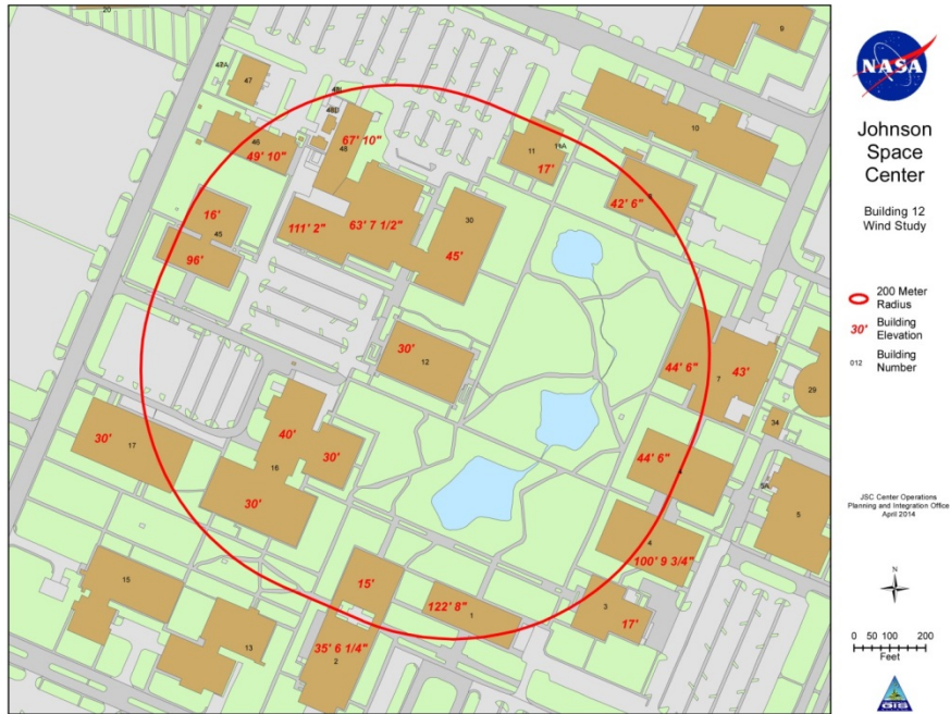
Figure 13. A part of the NASA Building 12 project assessment, this elevation map shows the height of surrounding structures.
