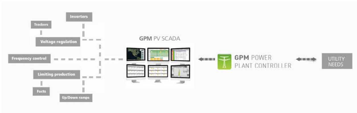
Figure 17. General diagram of a GPTech’s PPC
