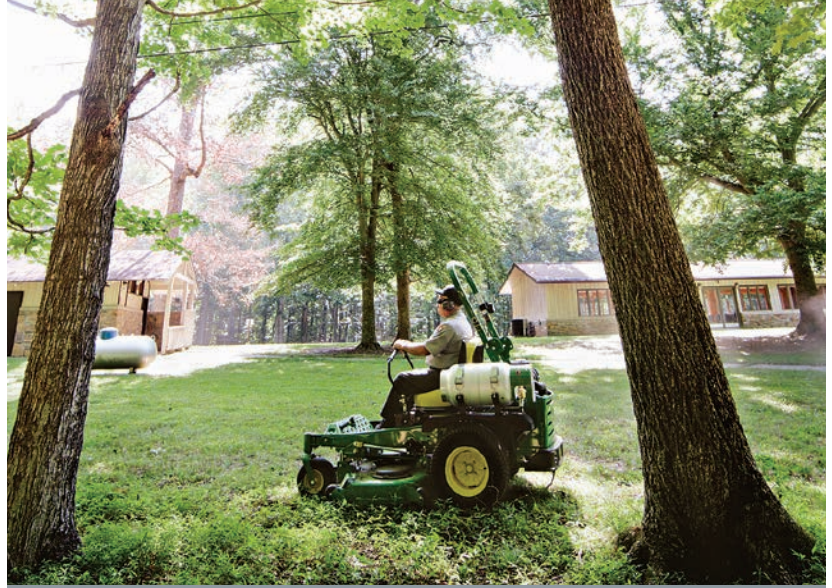
Propane mowers are cleaner burning than most gasoline or diesel mowers and may have reduced maintenance requirements. Photo from Geoff Johnson, PERC, NREL 31752
