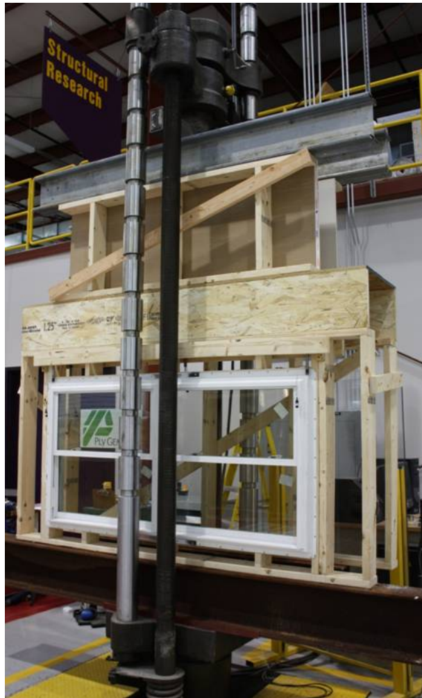
Figure 14. Advanced framing structural testing
