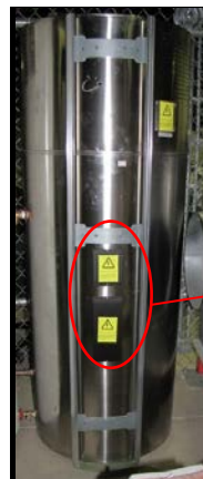
Figure 11. The AirGenerate HPWH with the heater covers shown.
