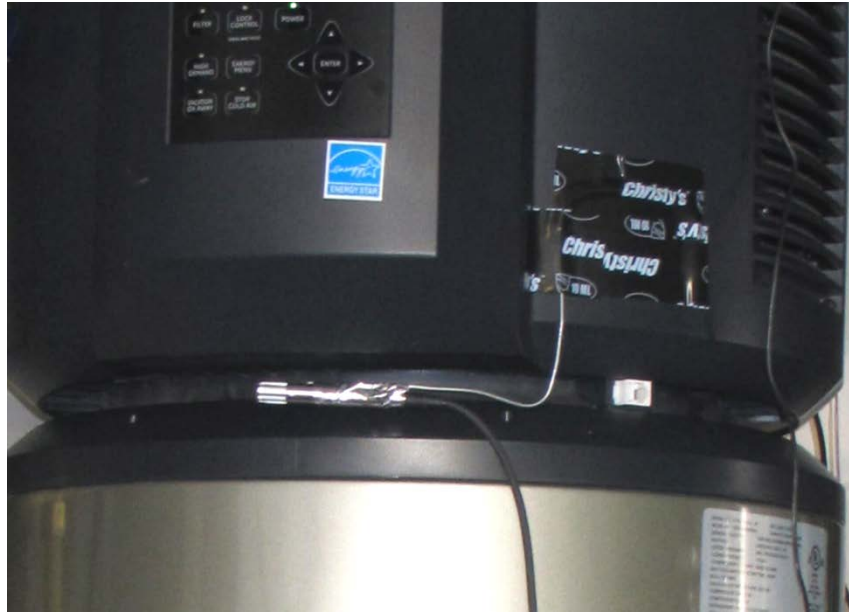
Figure 23. T&RH sensor is mounted on the front of the HPWH to measure inlet air conditions.
