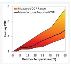
Chart of MSHP heating efficiency (COP) at various outdoor temperatures. The wide colored band represents efficiency variation due to different heating loads. The manufacturer's reported efficiency is indicated by the thick blue line.
