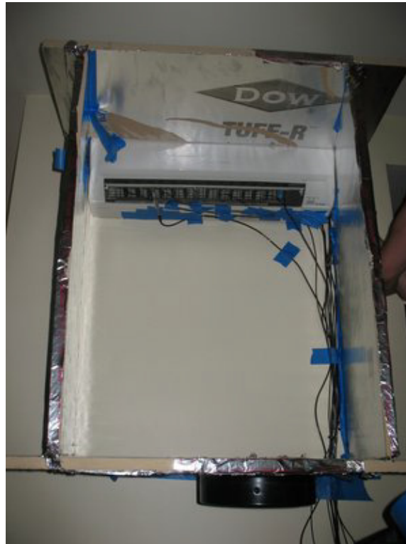
Figure 24. MSHP for indoor heat air flow test rigid plenum method
