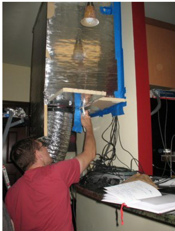
Figure 25. Researcher examining MSHP for indoor heat air flow test rigid plenum method
